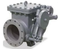
Therefore the (NON-SLAMMING check-valve) the next generation, such as the SCCV(Surge Control Check Valve) is developed based on an innovative concept, the SCCV mainly reduces the reverse flow velocity and deceleration without sudden stoppage of flow till the velocity becomes very low, resulting no slamming. on the other hand, the mass oscillation is being damped by the small Disc automatic controlled closure!
