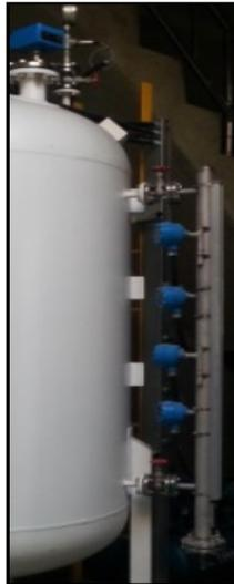
The credibility is improved with comparative logic control by the level switch in spite of a trouble with level sensor.
